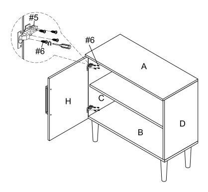
Step 8. Attach right door panel (part I) to right side panel (part D) using installed door hinges (part #5), small screws (part #6) and phillips head screwdriver.
