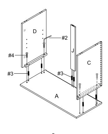
Step 4. Attach assembled unit (parts B & F) to assembled unit (parts A, C, D & J) using allen wrench (part #2), wood dowels (part #3), long bolts (part #11) and lock the hardware.
